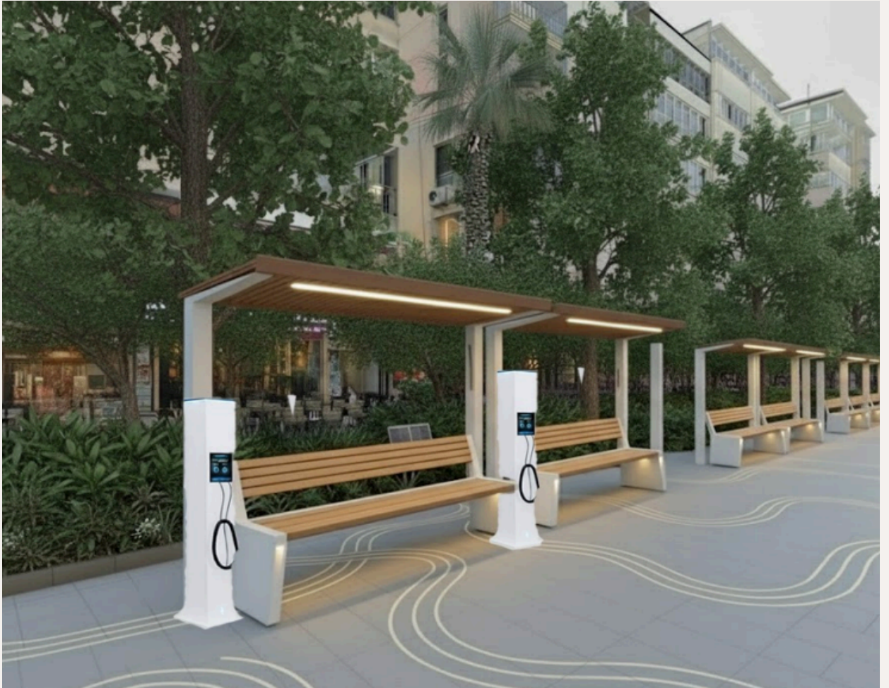
Figure 34. Photoluminescent road markings and vertical charging units
