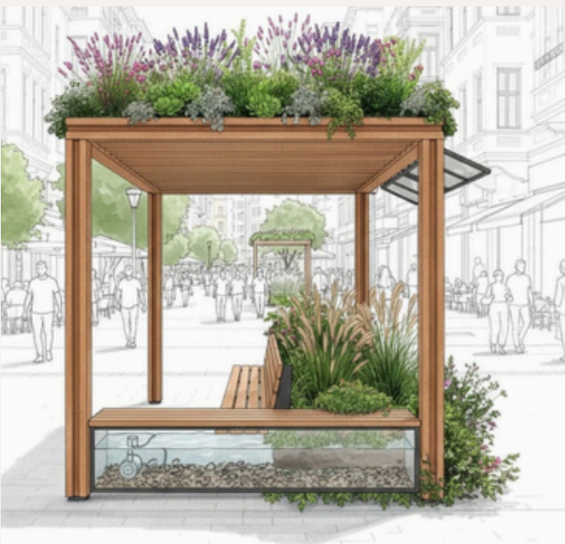
Figure 50&51. Green shading elements collecting rain water
