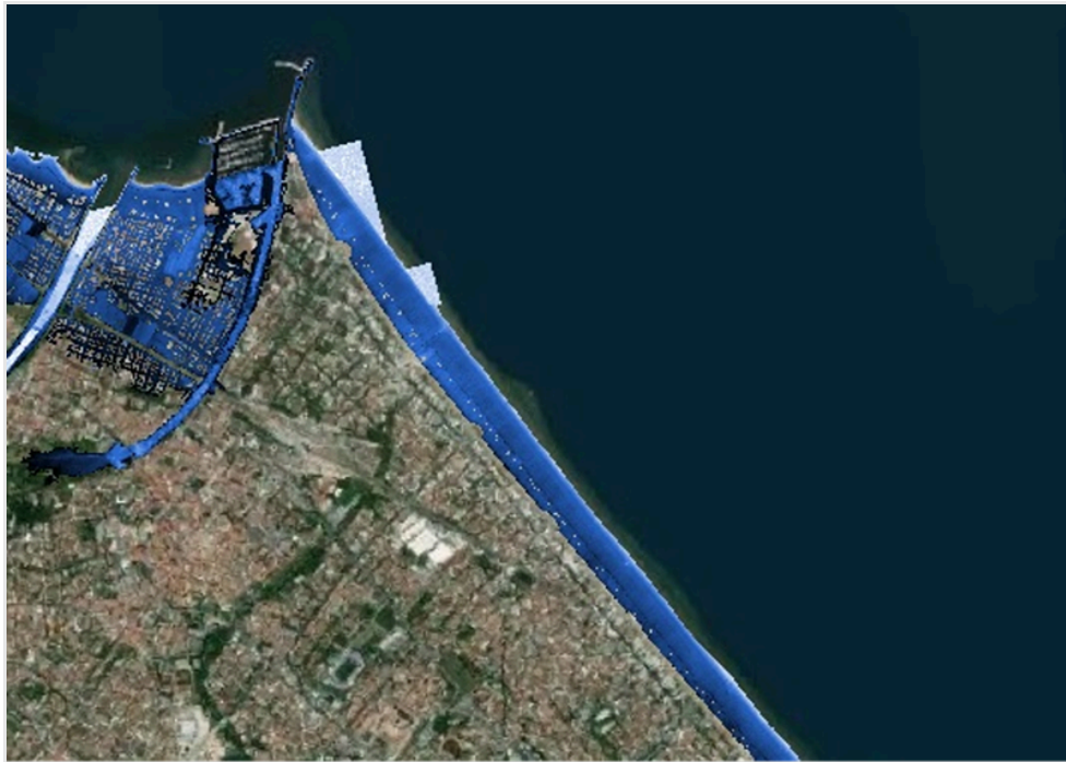
Figure 29 - Scenario at 2050 which represents the reduction of the city areas affected by the risk of flooding due to the elevation of the new waterfront created by the Parco del mare intervention.
