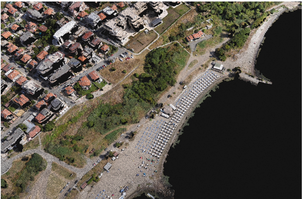
Fig. 24. Angled visualization of a 3D point cloud obtained from an aerial photogrammetric survey of the Project Territory – eastern part, Source: Sofia University “Saint Kliment Ohridski”
