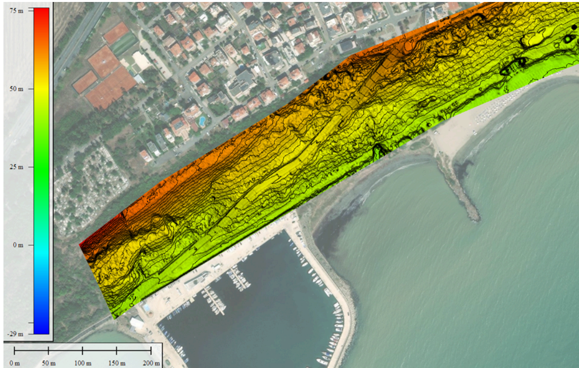
Fig. 26. Visualisation of laser scanning with LiDAR technology of the pilot territory, 2024, Source: Sofia University "Saint Kliment Ohridski"
